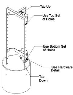
7 Assemble a screw with washers in the top mounting bracket. Leave the screw loose so the FRE-865 can be installed using its keyslot feature.
