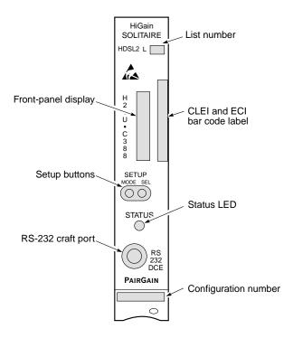
Figure 2. H2TU-C-388 List 1E Front Panel
