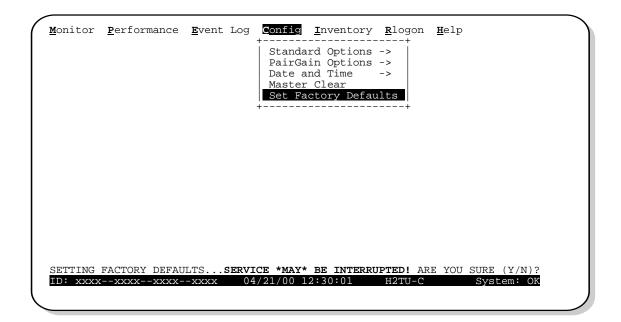
Figure 10. Configuration Menu - Reset to Factory Defaults
