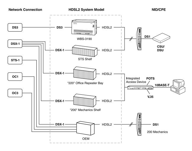
Figure 1. HDSL2 System Model
