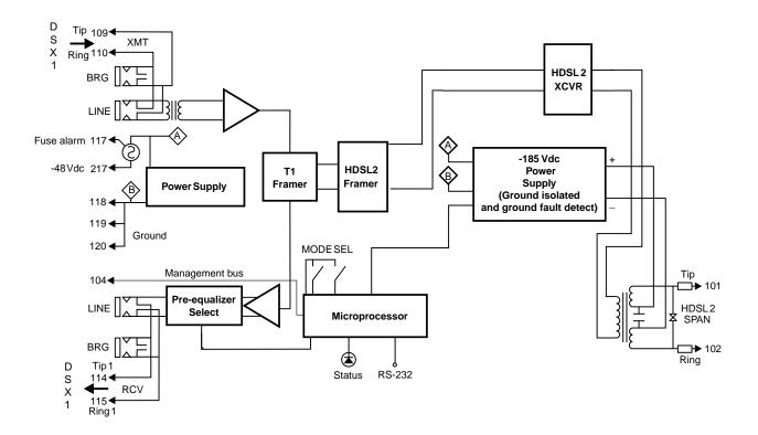
Figure 28. H2TU-C-388 List 1E Block Diagram Timing
