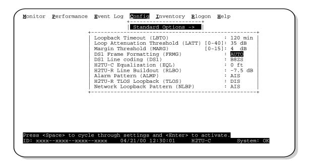
Figure 8. Configuration Menu - Standard Options (Defaults Shown)
