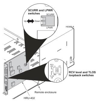
1 Set the DS1 RCV LEV and TLOS loopback switches. These switches set the DS1 receive line buildout level toward the Customer Interface (CI).
