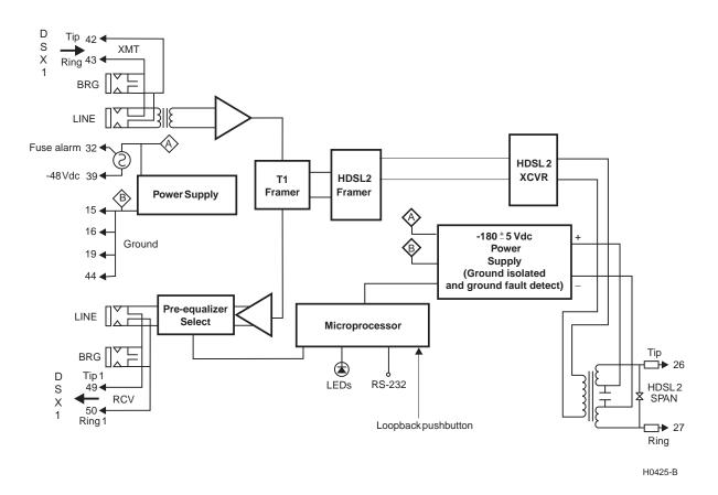
Figure 40. Block Diagram
