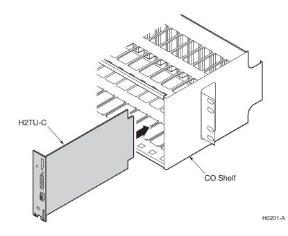
Figure 2. Installing the H2TU-C into a Shelf
