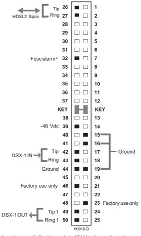
\* Fuse alarm is normally floating and at -48 Vdc when activated.\*\* Active pins are solid black.
