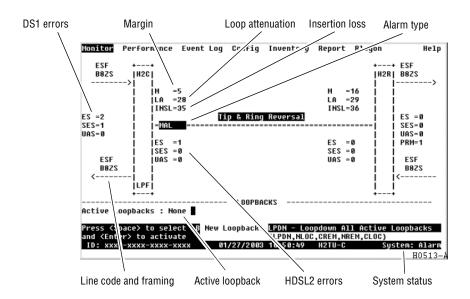
Figure 12. Monitor Screen - Active Loopback with Alarms
