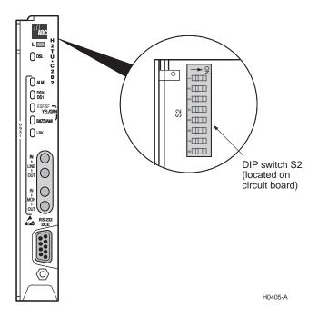
Figure 2. On-board DIP Switch S2
