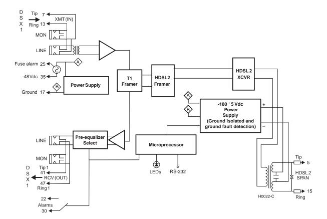
Figure 32. H2TU-C Block Diagram
