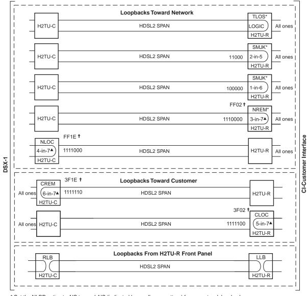
\* Set the NLBP option to AIS to send AIS (indicated by an all ones pattern) for any network loopback. H0033-A **†** A3LB loopback code.
