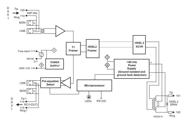
Figure 31. H2TU-C Block Diagram
