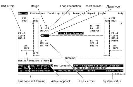
Figure 11. Monitor Screen - Active Loopback with Alarms
