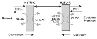
\* When enabled, TLOS is an automatic loopback that occurs with an LOS at the remote DS1 input.
