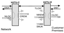
\* When enabled, TLOS is an automatic loopback that occurs with an LOS at the remote DS1 input.
