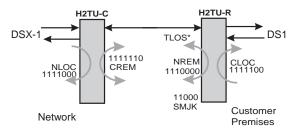
\*When enabled, TLOS is an automatic loopback that occurs with an LOS at the remote DS1 input.
