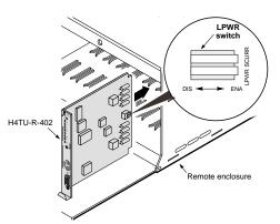
1 Set the S1 switches (SCURR and LPWR), located adjacent to the card-edge connector, as follows:
